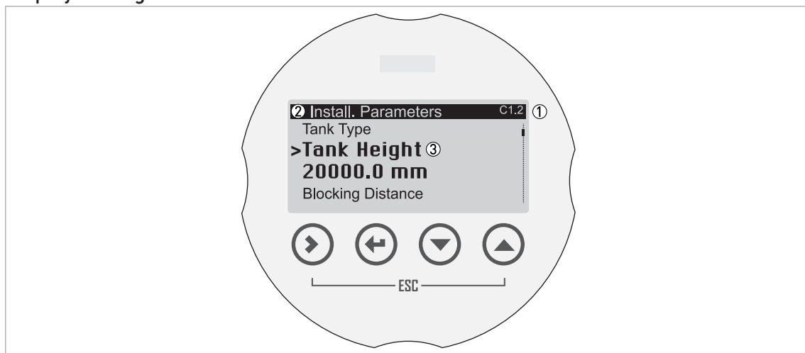
Figure 5-2: Display screen layout in Program mode
