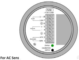
Power: 3 Wire unshielded 22 AWG, 300 V Hook-up Wire Current Output: 1 Pair shielded 24 AWG, 300 V Hook-up Wire
