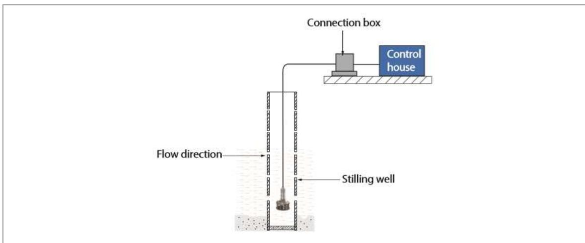
Fig.5. Installation in flowing liquid
