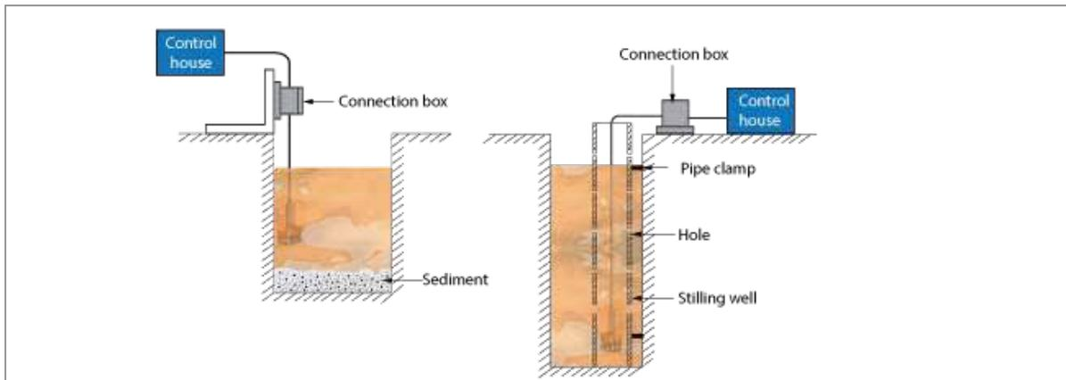
Fig.4. Installation in static liquid
