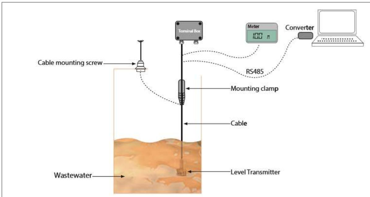
Fig.2. Mounting the transmitter
