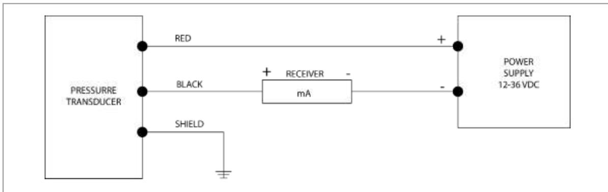
Fig.6. Power supply connections
